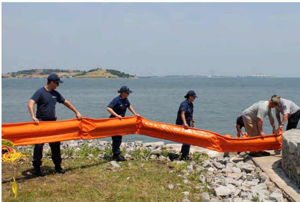
Figure 6. Deploying Boom from MITA Oil Spill Response Trailer
