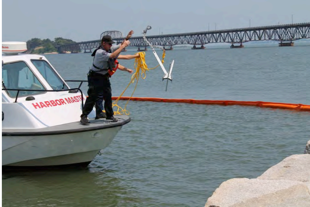
Figure 7. BPD First Responder Setting Anchor for Diversionary Booming Tactic
