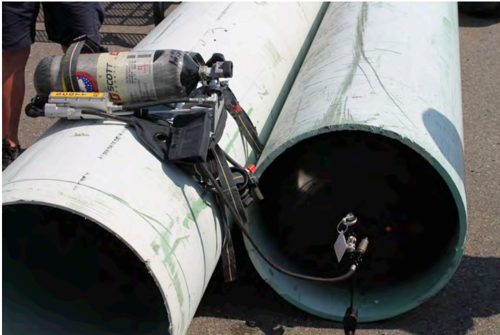
Figure 5. Culvert Plug Demonstration Using SCBA to Inflate
