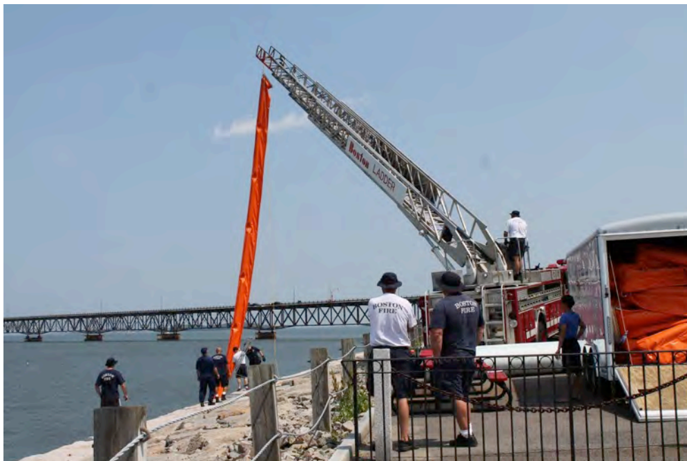
Figure 10. Demobilizing Boom Utilizing BFD (MITA) Ladder Truck
