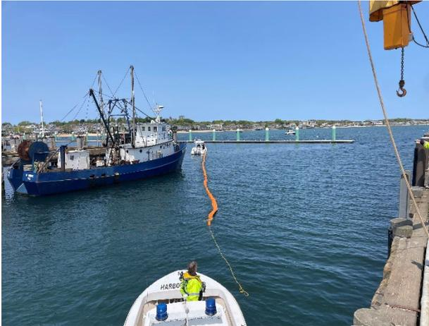
Vessel crews towing boom to the deployment site
