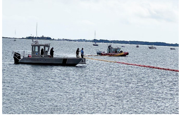
Vessel crews tow boom to the deployment site
