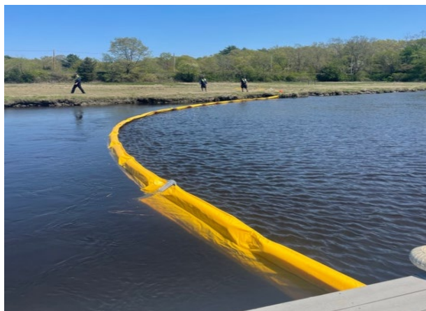
Figure 8: Crews finish reconfiguring DV01b to overcome tidal changes, then deploy peat moss to test the tactic
