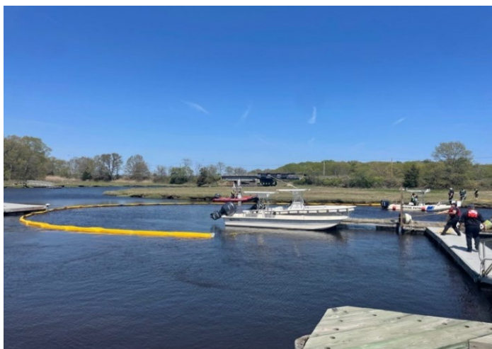
Figure 7: Shore and vessel crews deploy containment boom around a docked vessel
