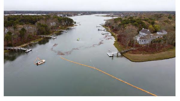
First responders deploy peat moss as an oil surrogate to test the deployed diversion boom configuration
