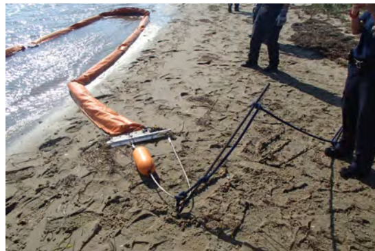
Bridle eye attached to first piece of rebar.
