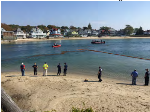
Boom captures surrogate (peat moss) with some evidence of entrainment due to strong current.
