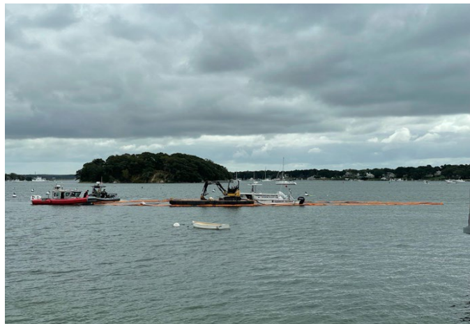
Figure 6: Crews position 300ft of boom around a vessel and barge at a mooring
