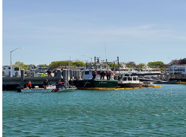
Figure 9: Vessel crews deploy 300 feet of boom around a fishing vessel in the harbor
