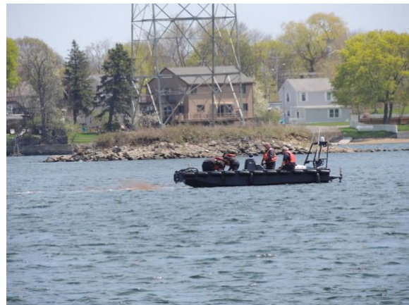
Salem Harbormaster personnel deploy peat moss as an oil surrogate to test the final configuration of the diversion strategy.
