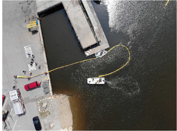
Vessel crews tow the second leg of boom towards the deployment site
