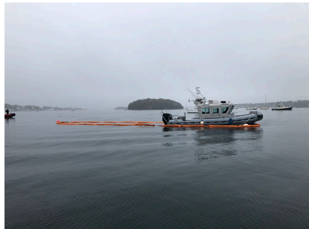
Containment boom around the anchored vessel successfully deployed.
