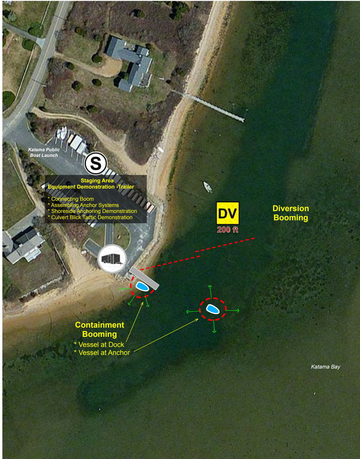
Figure 1. Containment and diversion booming tactics for Edgartown exercise.
