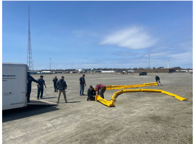
Shore team assembles the boom prior to deployment for a containment strategy
