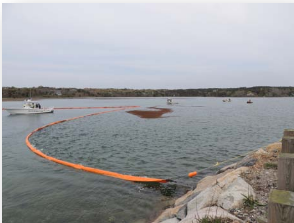
Oil surrogate (peat moss) is collected by boom in the Pamet River
